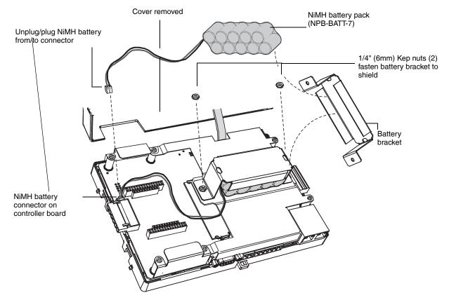
Fig. 12. Replacing NiMH battery pack in WEB/CP-700.
